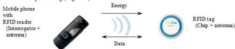
Figure 1. Mobile RFID system
